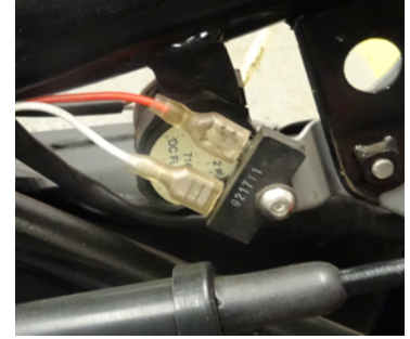
Rectifier: 2 wires, normally red and white. Mounted close to the HT coil.
