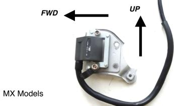
7. Connect the 'Hot' orange to the HT coil tag terminal.
