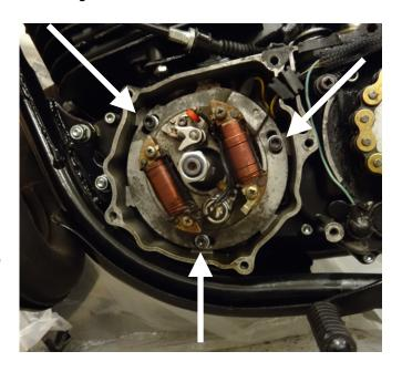
3. Fit the new stator with windings as shown. Ensure the three original threaded holes you removed the retaining screws from align with those in the new stator. Use the 3 x M6 c'sunk screws from the kit to retain the new stator. All 3 must be used. The stator will only align one way round with three screws in alignment. Securely tighten the screws.
