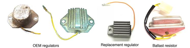
You must check in and around the headlamp, headstock and battery area for any of the above 6V components, if found they should be removed. Yamaha tried many different charging system configurations pre 1977 and it is now difficult to predict (on some models) what is fitted. It is also common to find one of these devices fitted by an owner in an attempt to stop bulb blowing. In this case these parts are often found mounted in unexpected areas.
