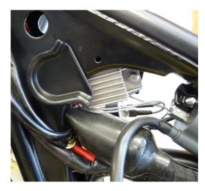
Plug in the new stator wire plugs in to the original wiring loom. Do not be alarmed if there is a different number of wires in the new stator plug or if they are slightly different colours, we have designed out kit to work on all of the different variations Yamaha created.
