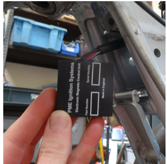
6. The CDI is adhered to the inside of the tool kit via the adhesive pad. Peel off the protective cover and stick to the inner RHS of the housing, with the wires positioned best to allow them to exit upwards.
