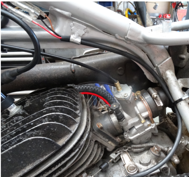
5. Route the stator wire up along the frame as shown. Cable tie it so it can't get caught by objects such as bushes or branches
