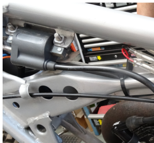
Correct HT coil mounting
