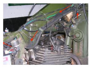
5. Follow the main loom round and connect the new green wire to one of the yellow wires on the regulator.
