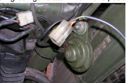
4. Route the new wire following the main loom as shown; use the cable ties to secure it so it does not chaff on the fuel tank.
