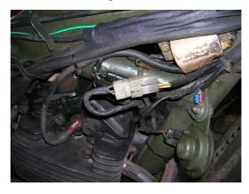
3. On the male side of the plug use your jeweller's screwdriver to release the green wire's tab from the housing, cut this wire backits no longer used. Fit the un-insulated tab on the new green generator wire in this position.
