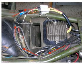
6. The purple & red T4 & T5 wires are not used, insulate them and tuck them away. Connect the regulator as shown on the connection guide. Reassemble the bike and test the charging IAW the maintenance manual
