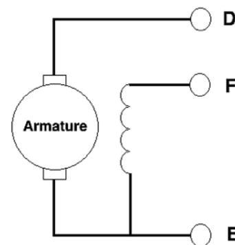
*The dynamo's internal connections must be as per all Lucas dynamos.*
