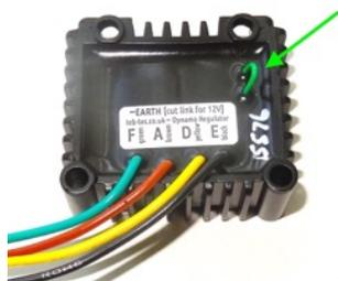
As supplied the regulator comes ready for 6 volt operation. By cutting the green loop wire the unit is converted to 12 volt operation. Cut the loop flush and apply a blob of epoxy glue over the cut ends to protect them.
