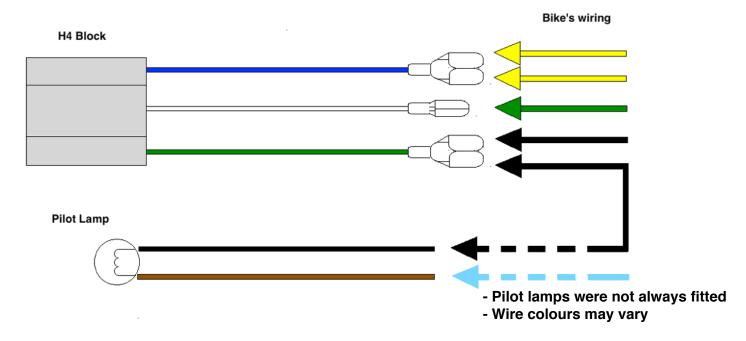
The above diagram shows how to connect Yamaha XT wiring to the H4 bulb holder in our kit that has standard European wire colours. Simply connect the bike's wiring to the new holder, matching up the colours as shown.
