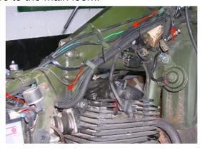
Refit the seat & fuel tank. Re-assemble the headlamp lens to the cowling.
