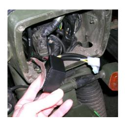
Feed the long leads through the back of the cowl. Connect the Molex connectors to the bike's loom and the bulb holder.
