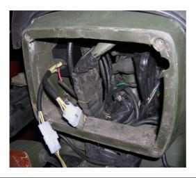
Remove the seat & fuel tank. Route the new lead following the main loom. Connect the red wire to the battery positive terminal and the black to the negative. Cable tie the new wire to the main loom.
