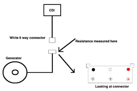
You are expecting a reading of 67 ohms +/-10%. If your meter isn't the "auto-ranging" type set it to a suitable ohms scale.
