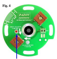
ANTI-CLOCKWISE ROTATION RED INDICATOR MARK ON MAGNETIC ROTOR ALIGNED UNDER ANTI-CLOCKWISE TIMING HOLE, ENGINE SET AT FULL ADVANCE
