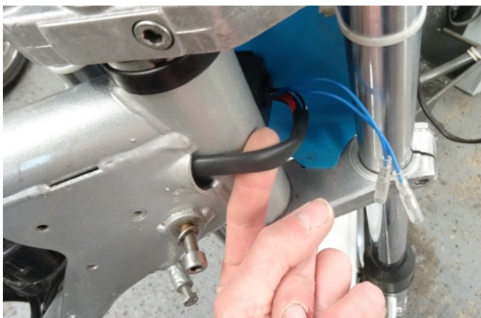
10. WARNING: Ensure you can easily slip one finger between the CDI wire and the headstock with the bars on full lock. If you cannot adjust the wires. Ensure the wires do not impeded the steering.
