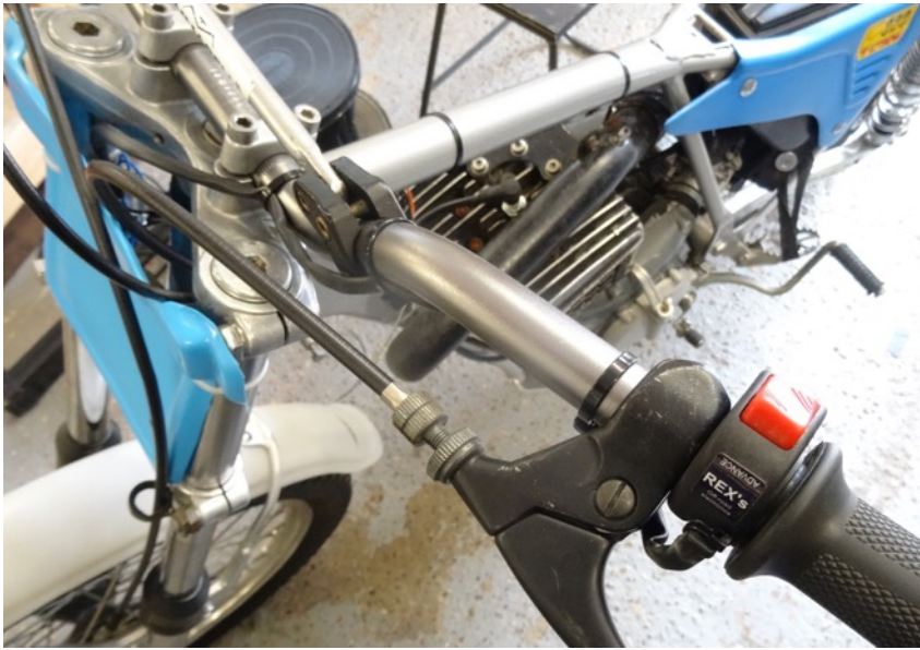
The switch will not fit to "fatbars" between the bar clamps.
