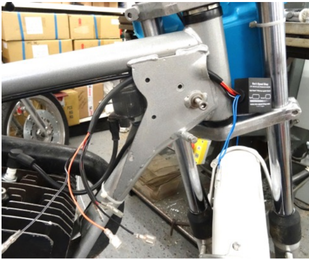
6. Route the wires from the CDI unit as shown
