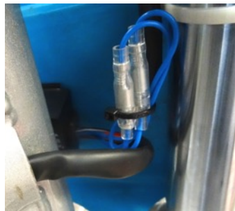
It does not matter which way round the blue wires connect. Secure the wires with a small cable tie.
