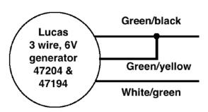
Earlier colours used by Lucas: light green, mid green & dark green wires. Join the mid and dark green wires for 12 volts.
