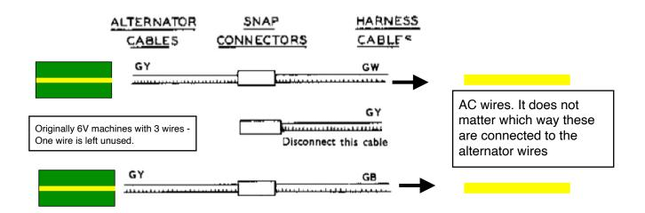
The DC connections to the new regulator rectifier are made at the rectifier DC connections. In fact if the machine has an ammeter, doing so ensures that the connections are made so that the ammeter shows a charge.
