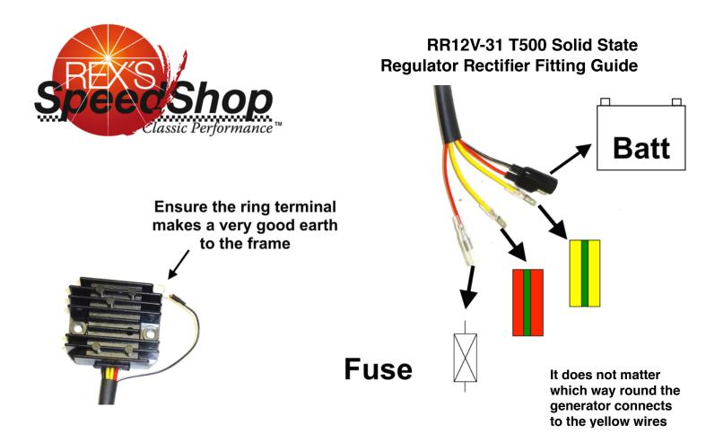
Our combined regulator/rectifier RR12V-31 is intended for T500 that had a separate regulator and rectifier units. It will automatically regulate the voltage if the lights are on or off. This unit can run with a lead acid, sealed, AGM batteries or battery-less, with our eliminator (part number BE1).
