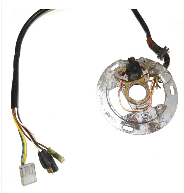
Lighting coil removed from stator (source coil also removed for rewinding)
