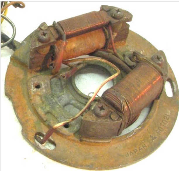
Auxiliary lighting winding above ignition source coil
