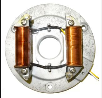
A lighting coil from a XT500. The lighting coil is the larger on the left when mounted on the engine. The TT lighting coil is in the same position, but is much smaller.
