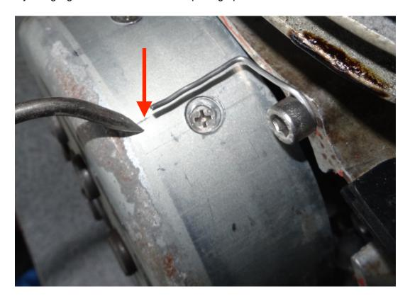
With the engine in the correct position, make a small scribe mark to correspond with the index
