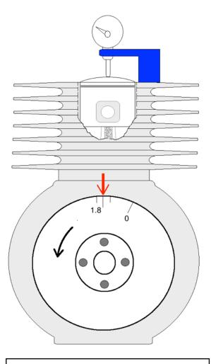
Once TDC is marked, make another mark for the static timing advance. Be careful to ensure you mark this BEFORE TDC and not after.
