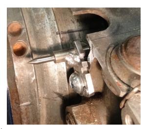
With the flywheel marked, mount the ignition kit as per the fitting guide. Use a strobe lamp to show the timing position. To adjust the static timing position the flywheel may have to be removed to access the the stator adjustment slots.
