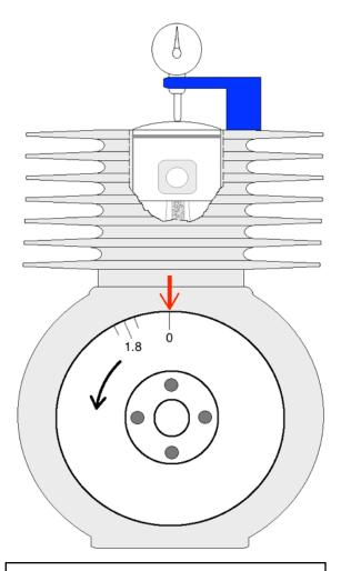
With the DTI suitably secured to the engine turn the crank in its normal direction of rotation until the piston reaches TDC. You will find that you have to over shoot and watch the DTI start to read in the opposite sense a few times before you find the exact point. When you are happy, zero the DTI
