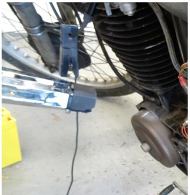
This is the point where the person tuning the engine has to decide where to set the timing according to how the engine responds. It could be that the stock figure remains suitable, in many cases the engine benefits from a slightly different setting. The engine tuner must use their skill to ensure the engine starts, idles and performs under load as intended while not allowing the ignition timing to become dangerous for the particular way the engine has been tuned.
