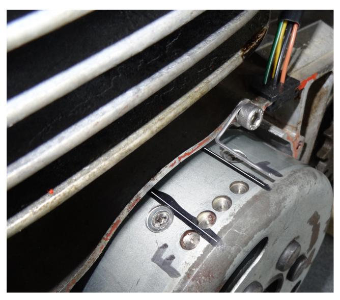
Flywheel now marked with a static 'F' mark and TDC. You can add extra marks either side of the 'F' mark, however there is no need to mark every degree. Every 2 or 5 degrees is usually sufficient. Make these marks shorter, so that the static mark remains clearly defined.
