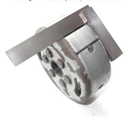
With the flywheel removed extend the small marks you made using a set square to ensure they are perfectly at 90 degrees to the edge of the rotor. It is vitally important to ensure the lines are at 90 degrees and do not 'wander' as this will reduce accuracy.
