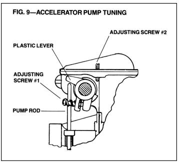
Figure 3: Accelerator pump stroke adjustor components
