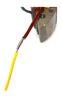
Shown (left) is a 'bootlace' splice, these are supplied in many of the universal hardware kits. Note kits for new 12 volt lighting coils will not have these if the wires come pre-attached to the winding. Universal kits contain the insulation, connectors, splices and a selection of useful hardware and electrical connectors.
