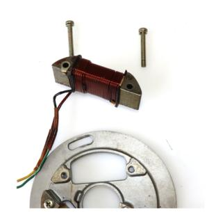
Cut the loom away from the stator, unscrew all the windings and separate the wires. Leave the 'tails' long ('tails' is the name for the solid wires coming from the winding).
