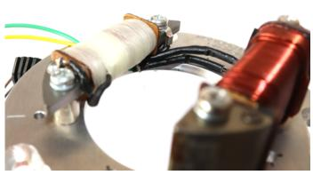
Caution: Where wires pass through a hole it is important they are protected with an over sleeve.
