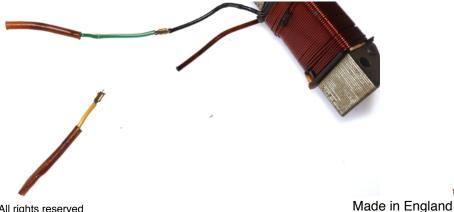
A craft knife can be used to scrape off the tough layer of enamel insulation from the magnet wire.
