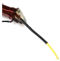
Slide a piece of high temperature sleeve over the heat shrink to protect the joint from heat and abrasion.
