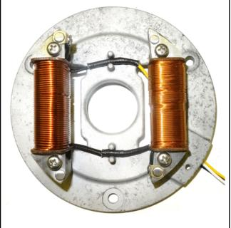
A lighting coil from a XT500. The lighting coil is the larger on the left when mounted on the engine. The TT lighting coil is in the same position, but is much smaller.
