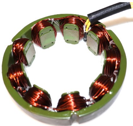
Radial stator - internal rotor with wound bobbins
