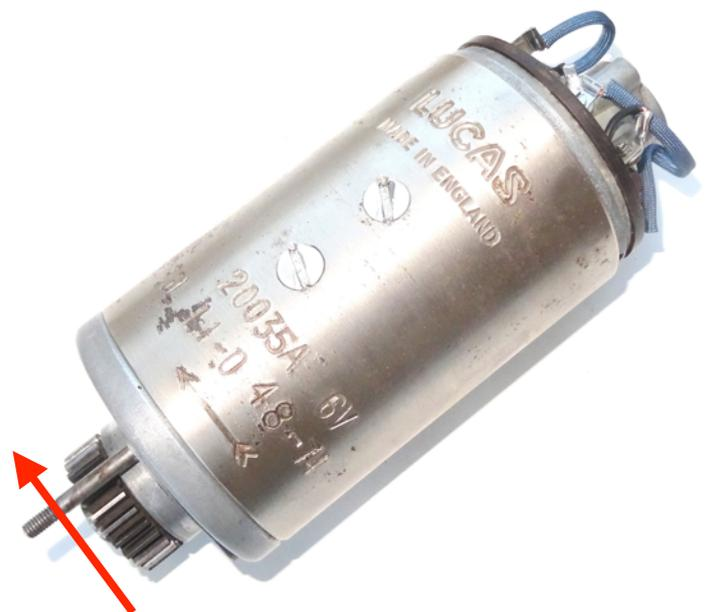
This is because the dynamo is a DC brush type motor that uses a field coil to produce the magnetic field. When a field coil is used, instead of permanent magnets, reversing the polarity of the battery does not change the direction of rotation. In order to change the direction the dynamo runs you have to change either the field coil connections or the armature connections. In our case it's a simple matter to reverse the field connections.
