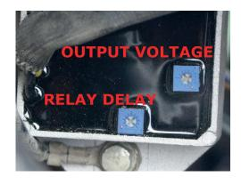
When mounted on the bike, the relay delay adjustment is on the bottom. The voltage adjustment is on the right. The adjustment procedure is as follows:
