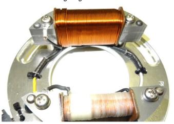
On LED windings both wires are yellow
