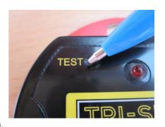
The spark plugs should begin sparking immediately at a rising rate for 10 seconds and then stop. The test can be repeated by pressing the test switch again. The LED should light during the 10 seconds while the system is sparking.
