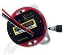
Loosely install the stator unit in the housing so that the holes for the pillar bolts are in the centre of the adjustment slots as shown here. Mark the housing with a pen next to the 'B' and then remove the stator unit.
