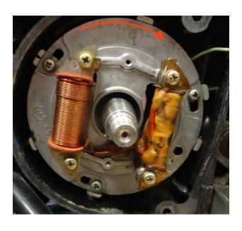
Normally turning the stator fully clockwise is enough to time the engine correctly. Owners who wish to experiment can elongate all 3 slots at the end shown nearest to the screws to give a larger range of adjustment.
