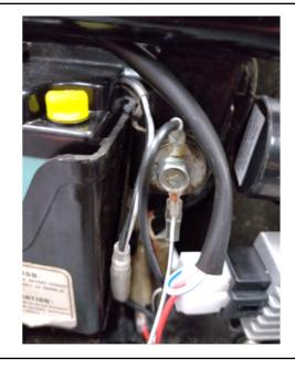
Wires in black sleeve - route over the battery, along the frame to the generator connections
