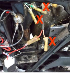
Locate and remove the rectifier and charge resistor, these are to the right of the battery.
