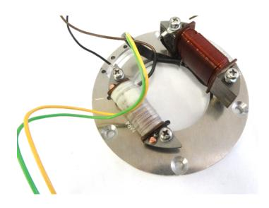
3. Remove the original generator case sealing grommet and combine the lighting wires in to the loom. Note these must go through the sleeve so they do not rub on the stator. Replace the cable tie and ensure the wiring is as close and flat to the stator as possible where it passes through it. Fit the new grommet.
