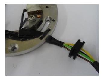
4. Combine the wires to the loom. Larger sleeve is included in the kit if the wires are too tight in the old sleeve. Fit male bullets as shown to the lighting wires. Replace the CDi connector (new one supplied). Ensure the wires match across the connector. Compare to the CDi connector!
