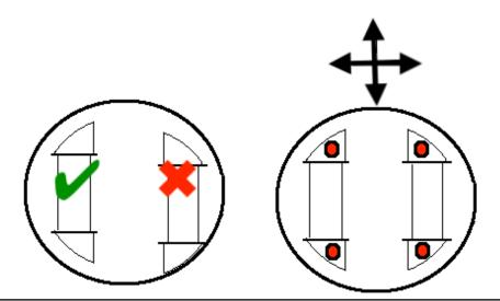
Use spring washers under the screw head and thread locking compound on the threads to avoid the screws becoming loose.
