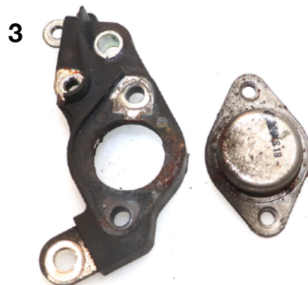
Regulator bracket. Connections 1, 2 & 3 are made to this. See line drawing below
