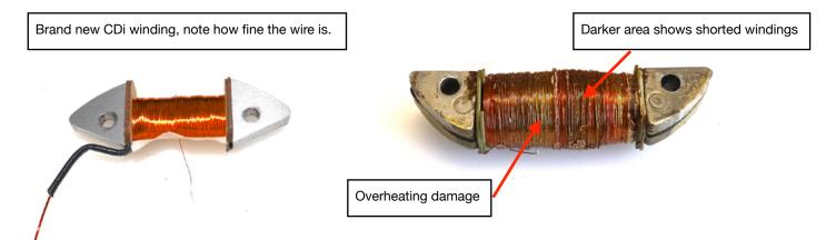
Electrical parts have precise specifications like mechanical parts have precision dimensions and these must be exactly right for the system to work. A poorly executed rewind that is off specification or still has the old insulation left in place often proves equally as problematic as an old winding.
