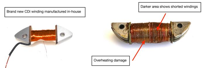
**Example.** The left source winding is brand new. The one on the right tested within the tolerances shown in the shop manual, leading the mechanic believe it was OK. Many parts were then replaced with worsening symptoms from the engine. Finally our technical team were contacted and parts sent for checking. The winding's top cover was removed to show damage to the windings that the resistance tolerance in the manual said was acceptable.
